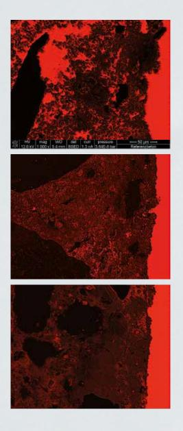
**Top: untreated concrete,** penetration of the resin indicates the original porosity of the cement paste that is relatable to the permeability of the paste.
